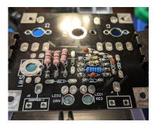
The case for the project is made from PCB's and is held together by soldering the corners and seams. This helps create a shielded case that is quite solid once completed.
